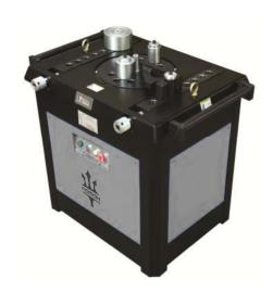
Bending machine used of customized Italian planetary gear box which is coupled with the motor, eliminates the use of "V" belts for reducing breakdown give higher torque and increases the productivity.
